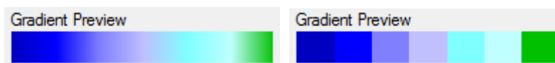
Fig. 7: Color gradient comparison of an interpolated gradient (left) and classified gradient (right), both based on the same thresholds
