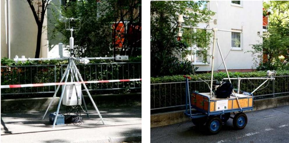
Fig. 3: Stationary (left) and mobile (right) human-biometeorological station used in the experimental investigation on human thermal comfort in Freiburg
