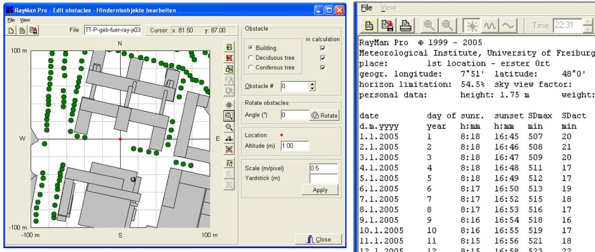
Fig. 2: Window for buildings and vegetation input (left) and data output for SVF and sunshine duration in RayMan
