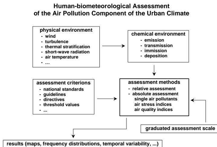
Fig. 3: Flow chart for the human-biometeorologically significant assessment of the air pollution environment
