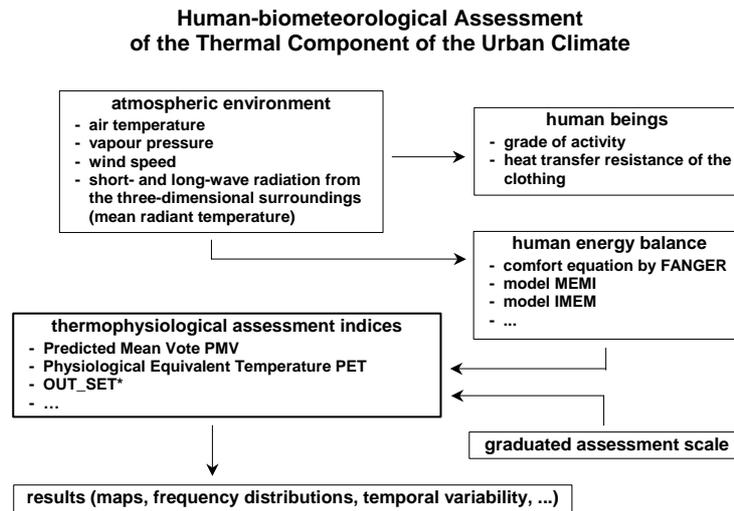
Fig. 2: Flow chart for the human-biometeorologically significant assessment of the thermal environment
