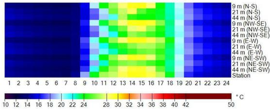
Fig 8. Diurnal Courses of Physiologically Equivalent Temperature (PET) (°C) for an urban canyon with north-south, northwest-southeast, east-west and northeast-southwest orientations, variable height (9 m, 21 m, 44 m) based on data from climate station for the period June 25th, 2003 to December 31st, 2010.
