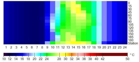
Fig 10. Diurnal Courses of Physiologically Equivalent Temperature (PET) (°C) for the stepwise (15°) rotation of an urban canyon with a height and width of 15m based on data from climate station for the period June 25th, 2003 to December 31st, 2010.
