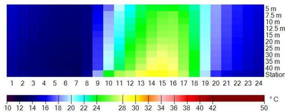
Fig 5. Diurnal Courses of Physiologically Equivalent Temperature ( $PET$ ) ( $^\circ C$ ) for an urban canyon with east-west orientation, 21m, height and variable width (5-40m) based on data from climate station for the period June 25th, 2003 to December 31st, 2010.
