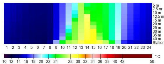
Fig 4. Diurnal Courses of Physiologically Equivalent Temperature ( $PET$ ) ( $^\circ C$ ) for an urban canyon with north-south orientation, 21m, height and variable width (5-40m) based on data from climate station for the period June 25th, 2003 to December 31st, 2010.
