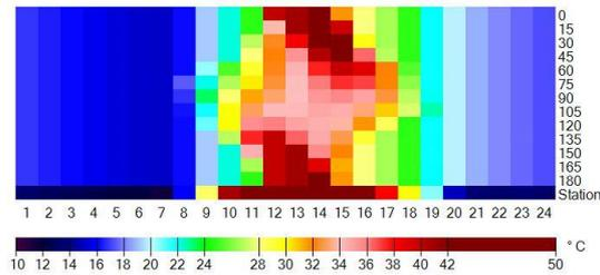
Fig 11. Diurnal Courses of Mean Radiant Temperature ( $T_{mrt}$ ) (°C) for the stepwise (15°) rotation of an urban canyon with a height and width of 15m based on data from climate station for the period June 25th, 2003 to December 31st, 2010.
