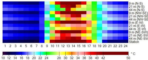
Fig 9. Diurnal Courses of Mean Radiant Temperature ( $T_{mrt}$ ) (°C) for an urban canyon with north-south, northwest-southeast, east-west and northeast-southwest orientations, variable height (9 m, 21 m, 44 m) based on data from climate station for the period June 25th, 2003 to December 31st, 2010.
