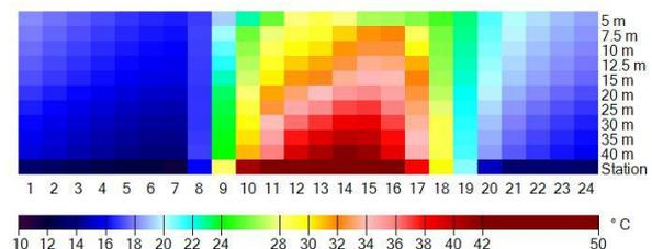
Fig 7. Diurnal Courses of Mean Radiant Temperature ( $T_{mrt}$ ) ( $^\circ C$ ) for an urban canyon with east-west orientation, 21m, height and variable width (5-40m) based on data from climate station for the period June 25th, 2003 to December 31st, 2010.
