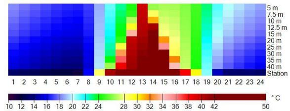
Fig 6. Diurnal Courses of Mean Radiant Temperature ( $T_{mrt}$ ) ( $^\circ C$ ) for an urban canyon with north-south orientation, 21m, height and variable width (5-40m) based on data from climate station for the period June 25th, 2003 to December 31st, 2010.
