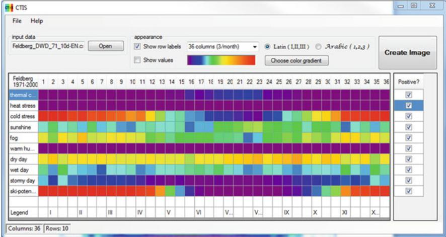
Fig. 3 CTIS main window for import of data, visual options and preparation of the factors (positive or negative)
