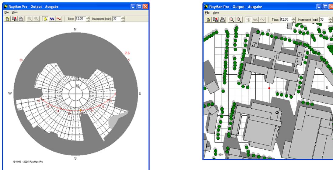
Figure 3: Example of sun path (left) and shade (right) on June 21 for a complex environment
