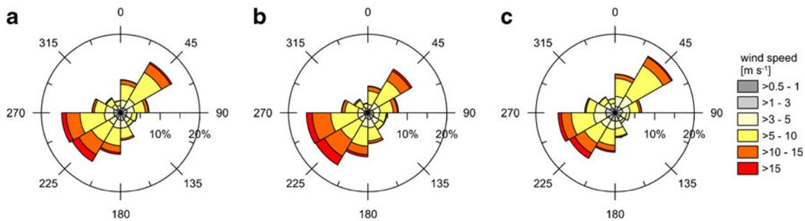
**Fig. 2** Wind rose for the airport station Findel based on hourly values for the period from 1986 until 2010 (excluding calms with wind velocity  $<0.5 \text{ ms}^{-1}$ ). *Left* figure (a) all values ( $N=203,431/\text{calms}=$
