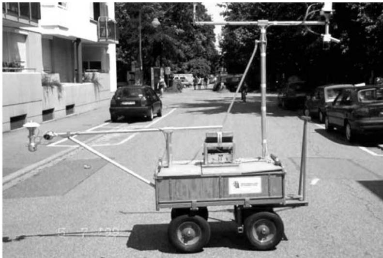
**Figure 1. Mobile human-biometeorological measuring unit (left: radiation sensors rotating around a horizontal and vertical axis to measure of the short- and long-wave radiation fluxes from the entire surroundings of a standing person)**
