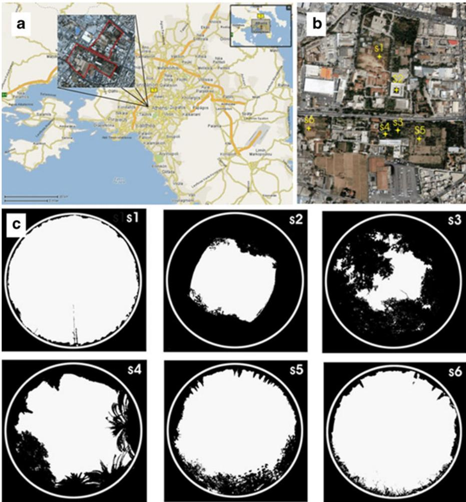
**Fig. 1** a AUA campus in Athens metropolitan area (b) Aerial photography of the selected sites in (c) The black and white fish-eye photography were used for SVF calculation at each selected site
